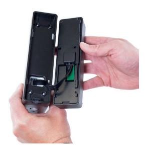
3. Detach the Control Head by disconnecting the cable between the Main Unit and the Control Head.
