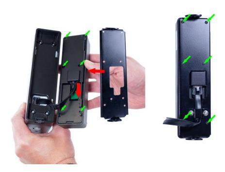
2. Connect the supplied 16 feet long RMK300 separation cable to the Control Head and install the supplied cable bracket to secure firmly the separation cable to the Control Head back cover.
