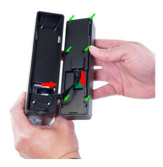
4. Remove the Control Head back cover by unscrewing the 6 screws pointed to with green arrows, as shown on the picture above (point 3).
