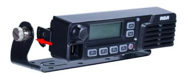
4. Mount the mobile radio Main Unit in the desired location and connect the other end of the separation cable to it.
